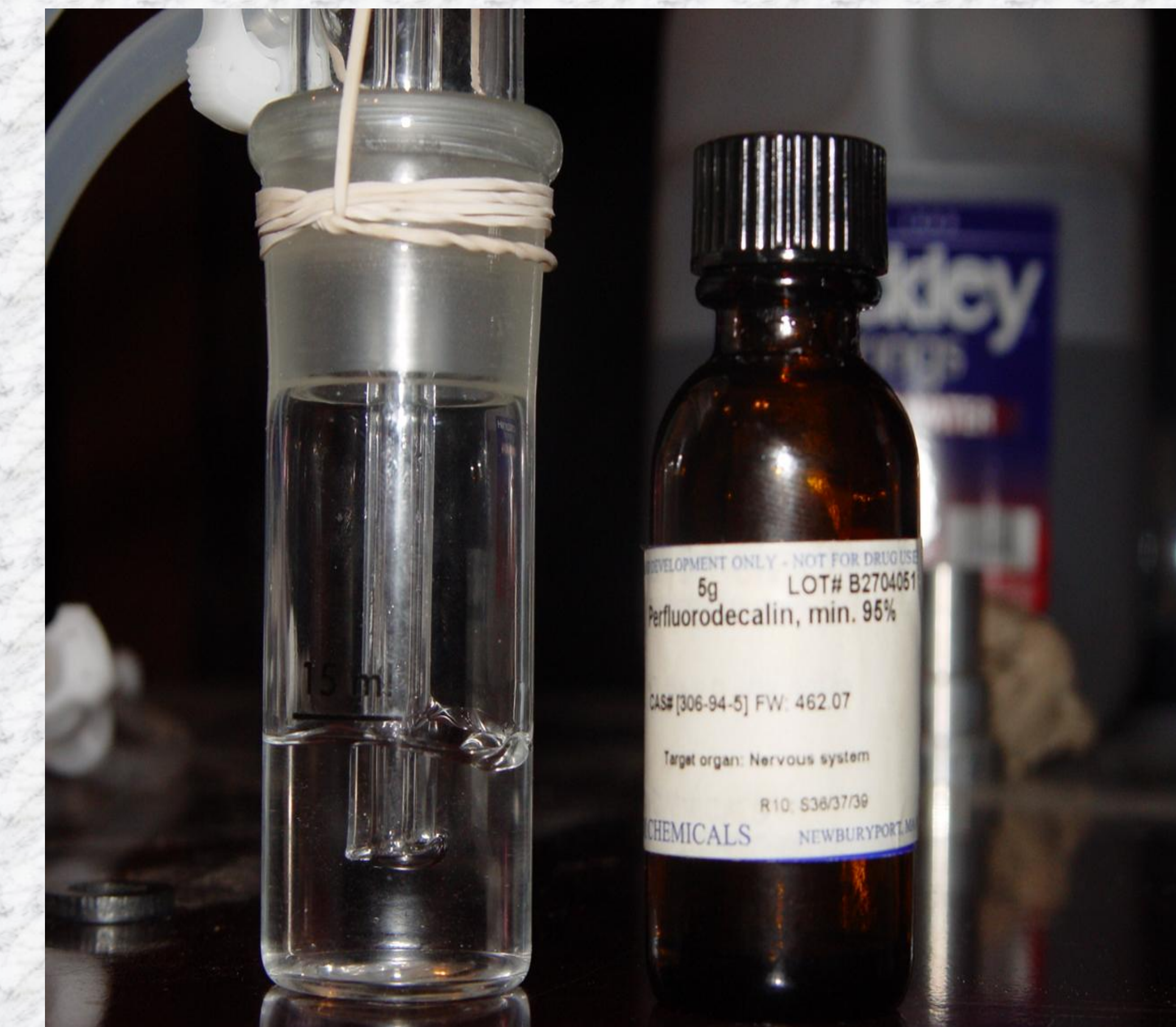
Bubbled Ozone gas for 25 min, then tested on Hatch DU 4000 spectrometer.
