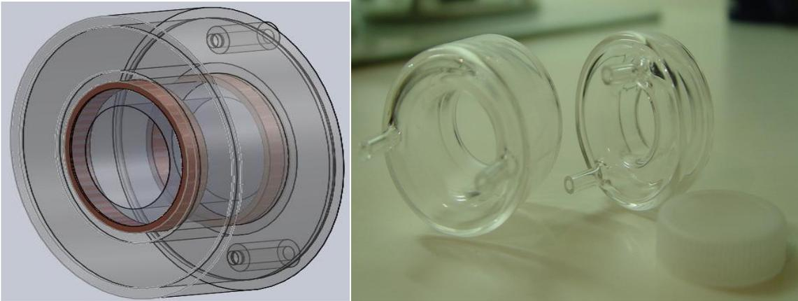
**Fig. 6:** Lamp design. Two competing bulb designs have been created.
