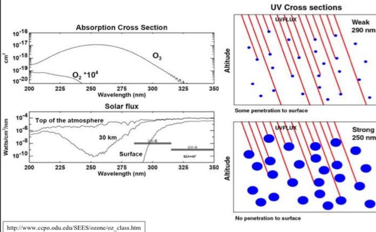
**Fig. 8:** UV absorption by O<sub>2</sub> and O<sub>3</sub> (7)
